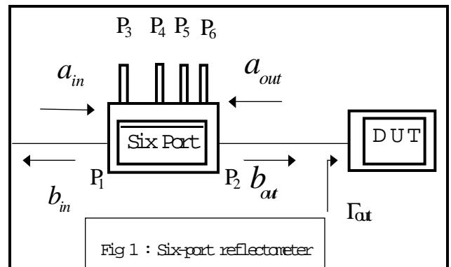
In the proposed configuration (see figure 2), incident and reflected waves  $a_{in}$  and  $a_{out}$  are completely independent and the six port junction reflectometer operated as a wave comparator providing the ratio  $a_{out}/a_{in}$ . This ratio as a function of the measured reflection
